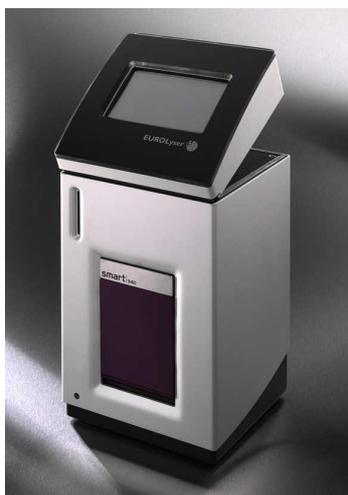
The Eurolyser *smart* laboratory photometer (figure 1) is an open measuring system, which means that various reagents from different producers can be applied. For measuring, the *smart* laboratory photometer is loaded with Eurolab reagent system (ERS) cassettes, in which the reagents of the particular producers are filled.
